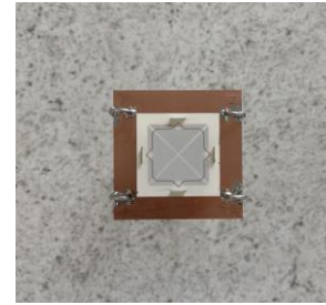
Fig. 15. Photo of the fabricated antenna element.
