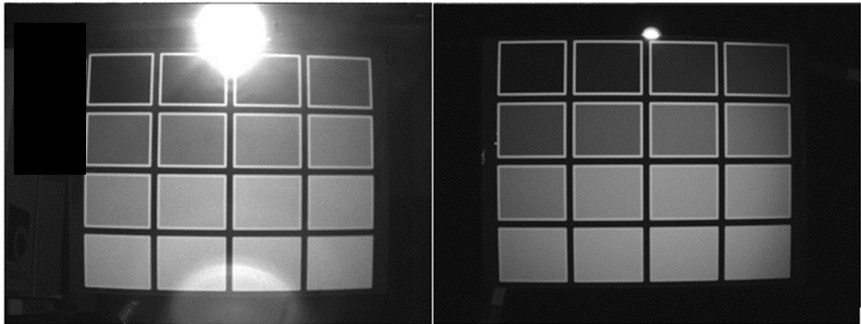
Figure 20 - Example of stray light in camera optical path and stray light mitigation.
