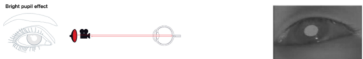
Figure 10 - Bright pupil detection system [16].
