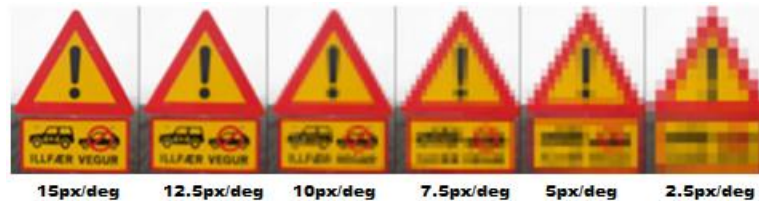
Figure 4 - Effect of decreasing resolution using the example of a traffic sign.
