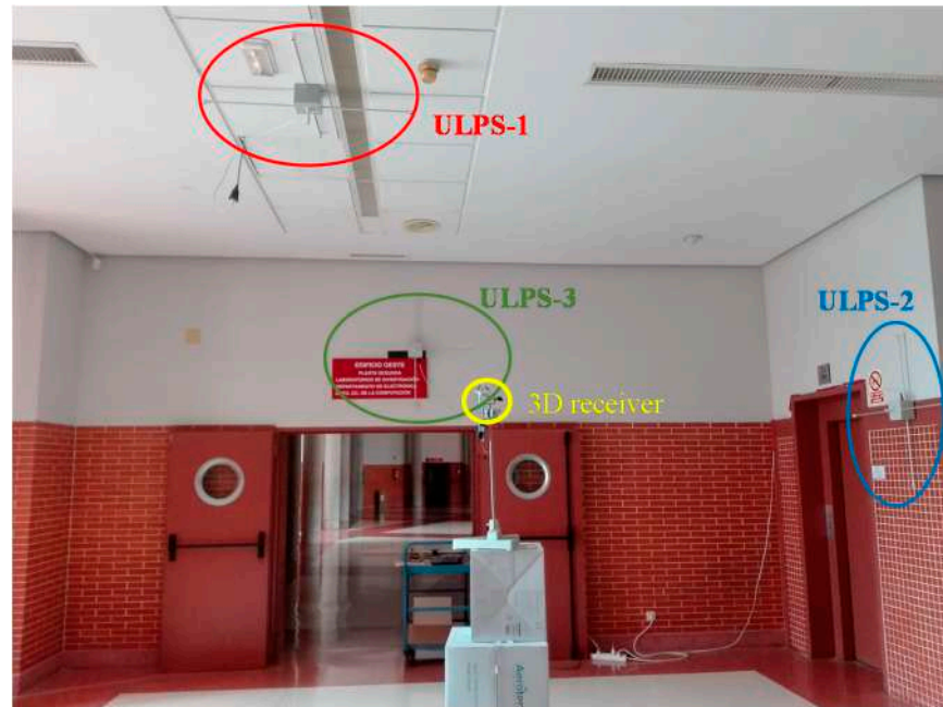
Figure 1. General view of the 3D scenario considered with three ULPS units installed on three perpendicular planes of the environment and a mobile receiver.
