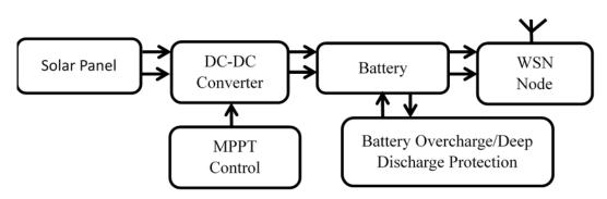
Fig. 2. Block diagram of solar energy harvesting system using PWM and MPPT control
