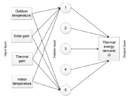
Fig. 4. Artificial neural network (ANN) architecture of building prediction model [42]
