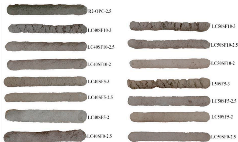
Fig. 4. Extrudability of LC3 mixtures with different limestone-calcined clay, SF and sand contents [59].
