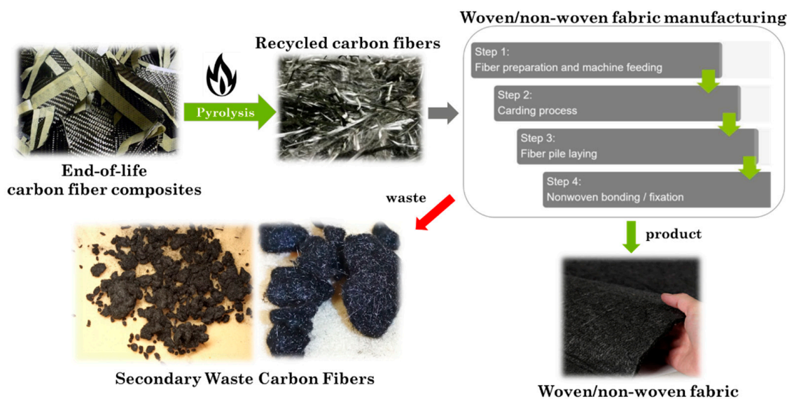
Figure 1. Flowchart of the process leading to the production of sCFs used in this work.
