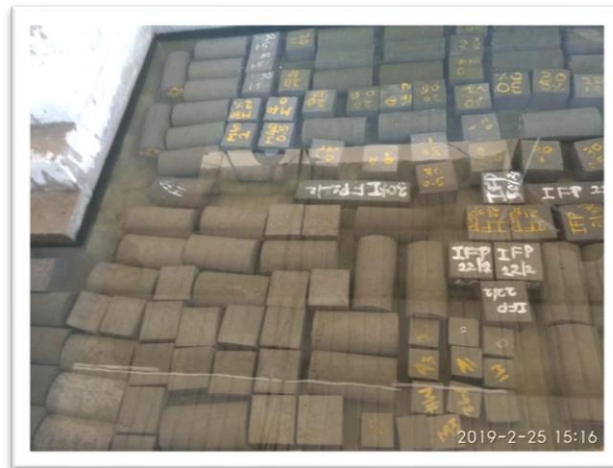
Fig. 3. SPECIMENS UNDER CURING FOR ALL CONCRETE MIX DESIGN
