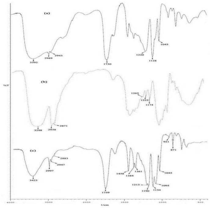
Figure 2. FTIR spectrum (lactic acid); (b) 1,4-butanediol; (c) PLA-OH
