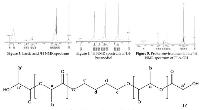
Figure 6. Structure of synthesized PLA-OH
