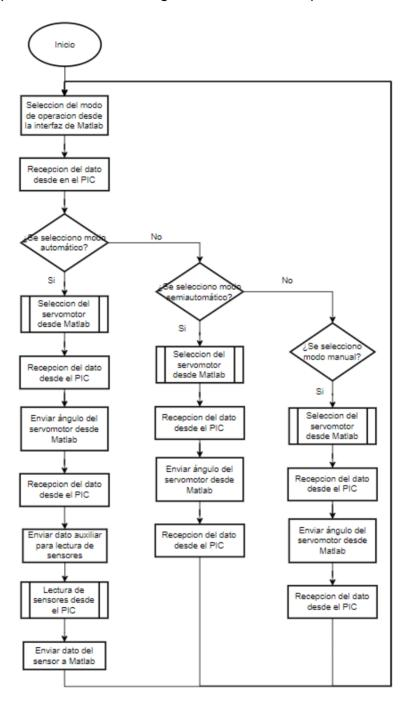
**Figure 5.** Flowchart for code implementation in Mplabx - (a) Selection of the operation mode and (b) distinction of the presence sensors.
