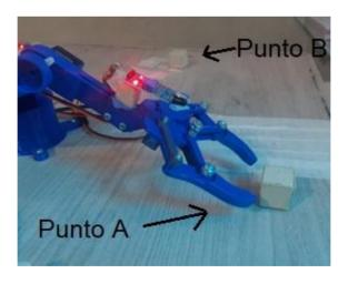
The semi-automatic mode works by means of the equations of the inverse kinematics of the 3R robot, with the purpose of entering a vector with X, Y and Z coordinates by keyboard through an HMI interface, so that the robot advances and positions the end effector in that coordinate entered by the user, as long as it is within the range of the robot, that is, in the work area.
