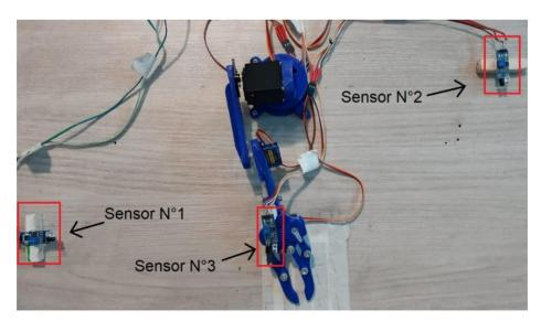
**Figure 14.** Sensors attached to the 3R robot.
