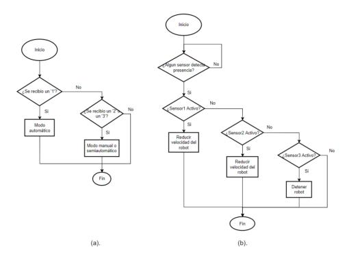
Figure 6. Flowchart for code implementation in Mplabx - Servomotor selection.
