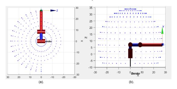
Figure 8. Work area of the 3R robot isometric view.
