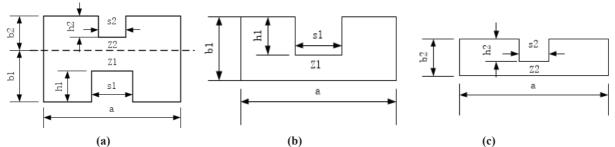
Figure 1 The asymmetrical double ridge waveguide. (a) Top view, (b) left-side view, and (c) right-sight view.
