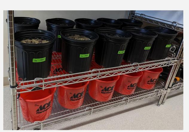
Figure 1. Experimental setup for nitrate leaching and water sample collection. The black pots on the top shelf contain roots and soil leftover after shoot biomass was collected. The red buckets on the lower shelf were aligned below each pot to collect water that leached through the soil. These water samples were frozen and analyzed for nitrate content. Image credit: Madelyn Schoenberger
