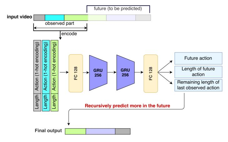
Figure. 1. Architecture of the RNN system [4]
