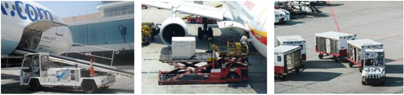
Fig. 1. Ground handling equipment (from left: belt conveyor, scissor lift, tractor with cages)
