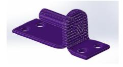
Fig. 15. Sliced door hinge model by layers in SolidWorks.
