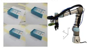
Fig. 2. The location of four points  $SP_1$  (0, 0, 0),  $SP_2$  (10, 0, 0),  $SP_3$  (0, 10, 0), and  $SP_4$  (0, 0, -10) of the packed salt object and the coordinate system of the robot used in the experiments.
