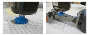
Fig. 9. Grasping of (a) washer and (b) drill with vacuum gripper.
