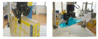
Fig. 6. Grasping of cereals box (a) and glass cleaner (b) with the two-fingered gripper.
