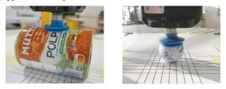
Fig. 8. Grasping of (a) tomato can and (b) golf ball with vacuum gripper.
