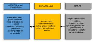
Fig. 14. Shematic of ADAMS/MATLAB co-simulation model.
