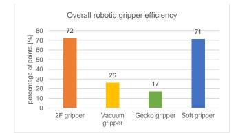
Fig. 4. Overall robotic gripper efficiency for selected objects.
