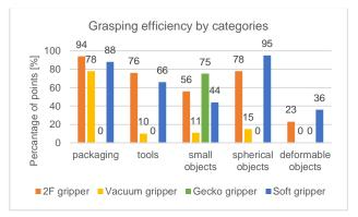
Fig. 5. Grasping efficiency of the robotic gripper by categories.
