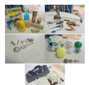
Fig. 1. The proposed five categories of objects to be grasped from the original YCB Gripper Assessment Protocol.
