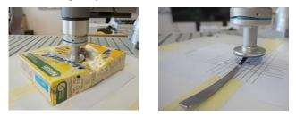
Fig. 10. Grasping of the (a) cereals box, and (b) spoon with the gecko robotic gripper.
