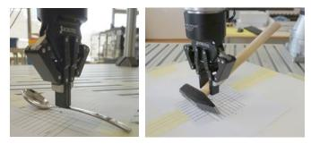
Fig. 7. Grasping of (a) spoon and (b) hammer with the two-fingered robotic gripper.
