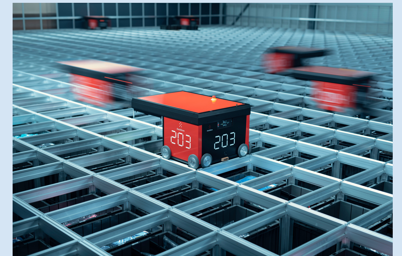
The AutoStore system as an example of grid-based motion planning in a bin storage application ©AutoStore
