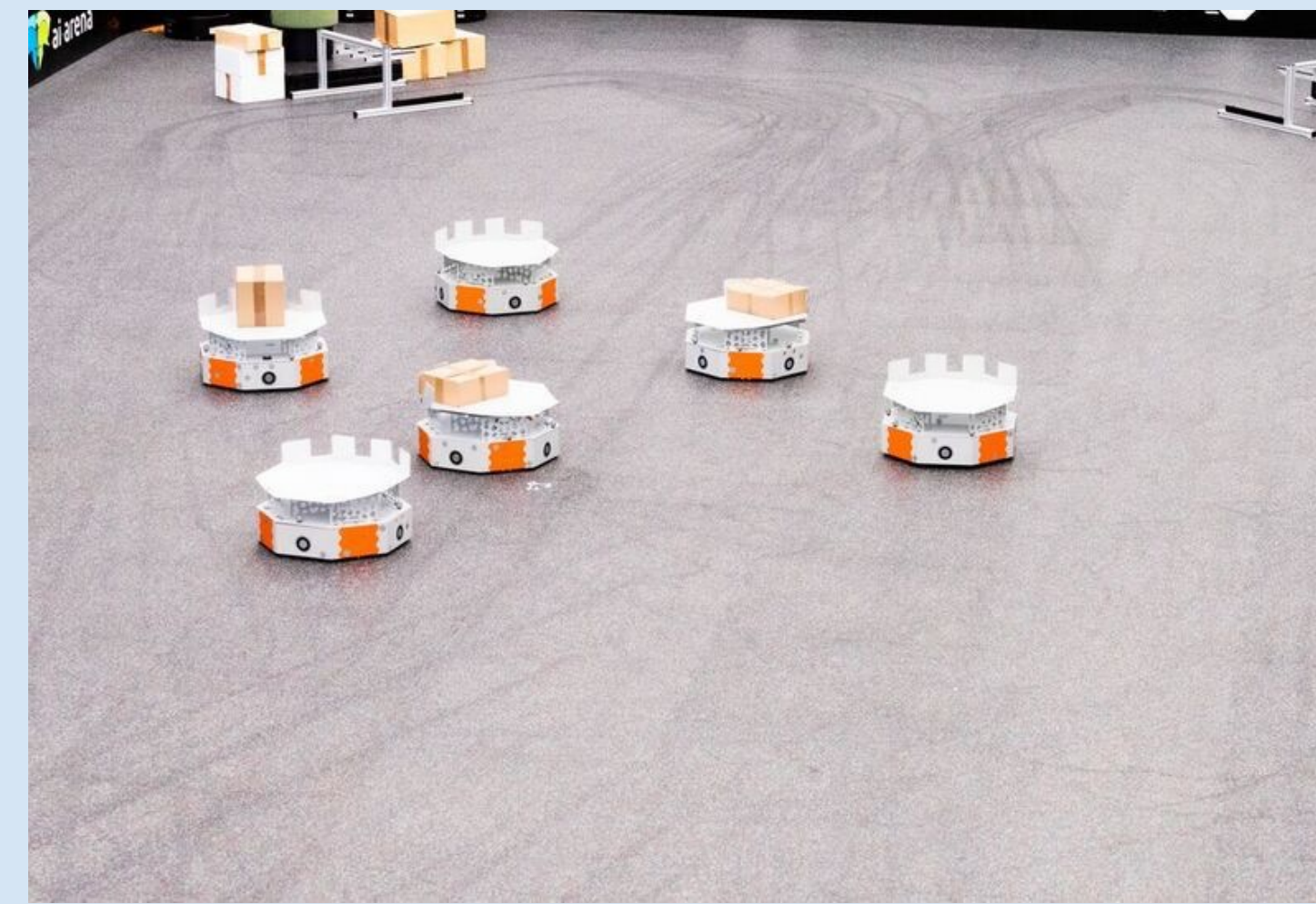
The Loadrunner as an example of free-form motion planning in a packet sorting application
