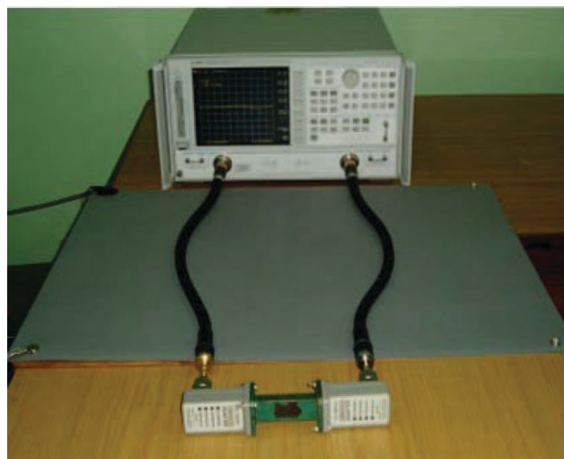
Figure 1 Experimental set-up for the measurement of complex permittivity and complex permeability. [Color figure can be viewed in the online issue, which is available at wileyonlinelibrary.com]
