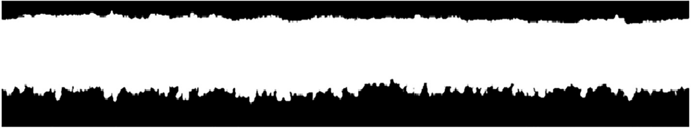
Fig. 1. Binary image of the cross section of the signal trace of black oxide VLP foil on PPO blend substrate.
