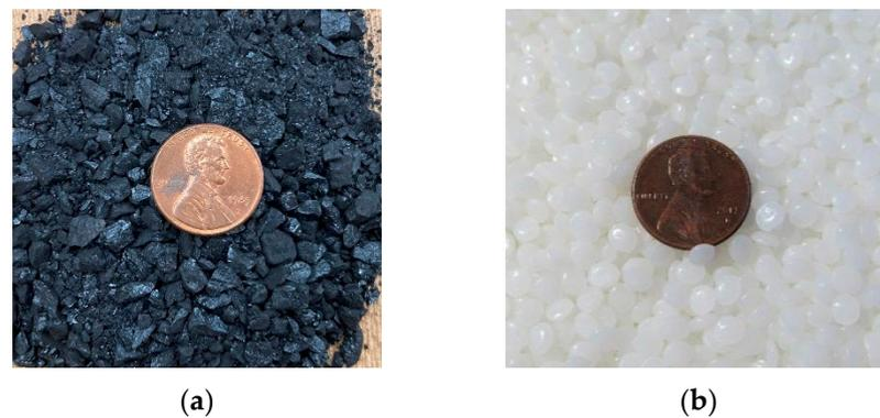
**Figure 1.** Sample of (a) bituminous coal and (b) recycled HDPE granules.
