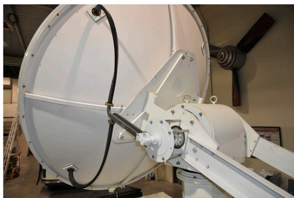
FIG. 17. This rotary joint is more robust than the original flexible waveguides. All XPOL units have been upgraded after the IFloodS campaign to operate with the rotary joints.
