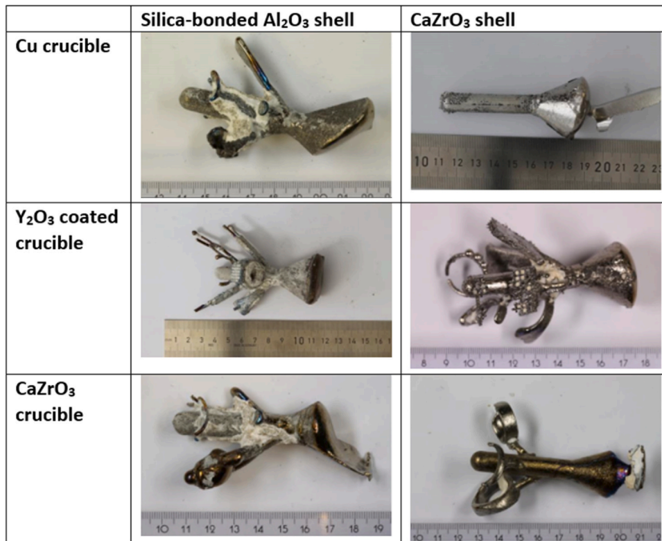
Fig. 18. A comparative analysis of different crucible and mold materials to optimize the properties of Ti-6Al-4V castings. The used crucibles were water-cooled copper, yttria and calcium zirconate respectively, while the investment molds were made of a commercial silica-bonded alumina shell and a calcium zirconate shell. The best combination was the water-cooled copper crucible and the calcium zirconate shell mold (recreated with permission from Ref. [29]).
