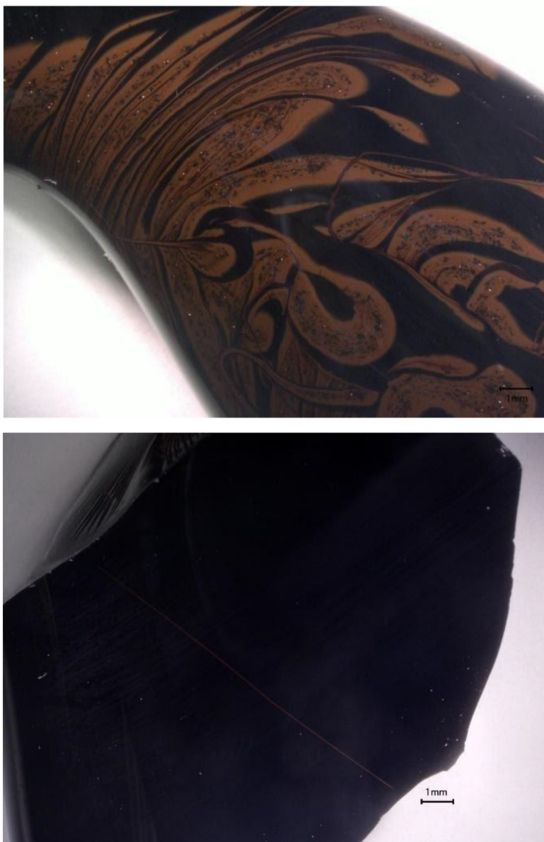
Fig. 7. Photograph of IL-03 glass after the viscosity measurement: (a) top portion of the quenched glass; (b) the bulk glass ( \geq 80\% of volume) after measurement.
