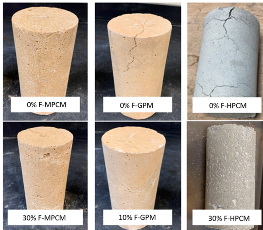
Fig. 11. Representative image of cracking.
