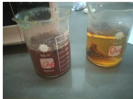
Figure 3: Effect of adding Hydrazine hydrate on Iron and chitosan solution
