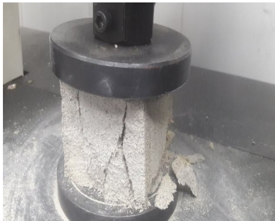
FIGURE 3 SHOWS CEMENT BRICK WITH POWDER USED TIRE AFTER COMPRESSION TEST
