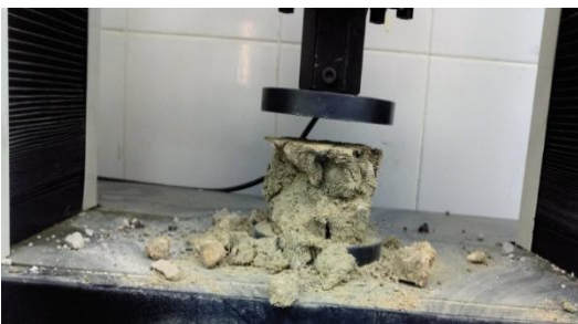
Figure 2 Cement brick with rice straw and glass powder addition after applying compression test
