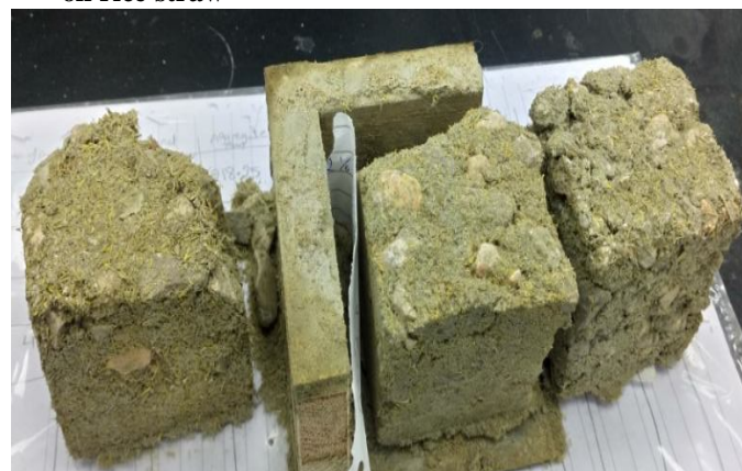
Figure 8 Three different percentage of rice straw added to Cement brick 1:2:2 ratio consists of: cement, sand and aggregates
