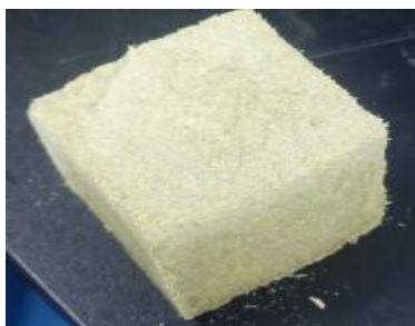
Figure 5 Cement-Sand Brick of rice straw based
