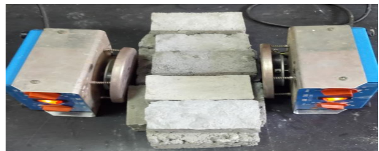
Figure 10 Thermal insulation test of cement bricks of ratio 1:2:2 by Ex-tech 5-in-1 Environmental meter
