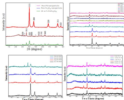
**Figure 3.** (a) XRD patterns of Pd, Fe<sub>3</sub>O<sub>4</sub>, and 20 wt% Pd/Fe<sub>3</sub>O<sub>4</sub> prepared using 0.4 ml hydrazine hydrate. (b, c, d) XRD patterns of 20 wt% Pd/Fe<sub>3</sub>O<sub>4</sub> prepared using different hydrazine hydrate ratios. (\* is due to Fe<sub>2</sub>O<sub>3</sub>).
