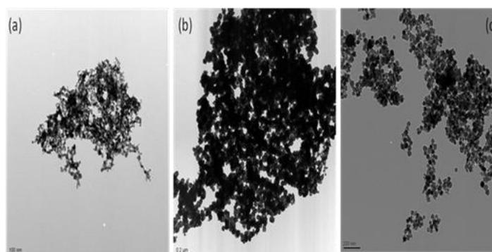
**Figure 2.** TEM of nanoparticles of: (a) Pd, (b) Fe<sub>3</sub>O<sub>4</sub>, (c) Pd/Fe<sub>3</sub>O<sub>4</sub>.
