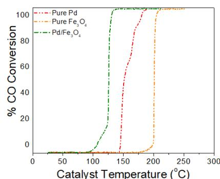
**Figure 5.** CO catalytic oxidation by 20 wt % Pd/Fe<sub>3</sub>O<sub>4</sub> with pure Pd and Fe<sub>3</sub>O<sub>4</sub> nanoparticles.
