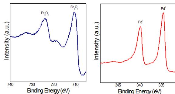
**Figure 4.** XPS binding energy of (a) Fe 2p region (b) Pd 3d region for Pd/Fe<sub>3</sub>O<sub>4</sub>.
