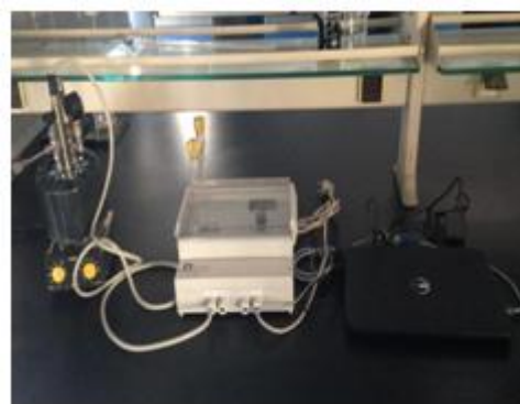
Figure 4. Open Cup Flash Point Test
