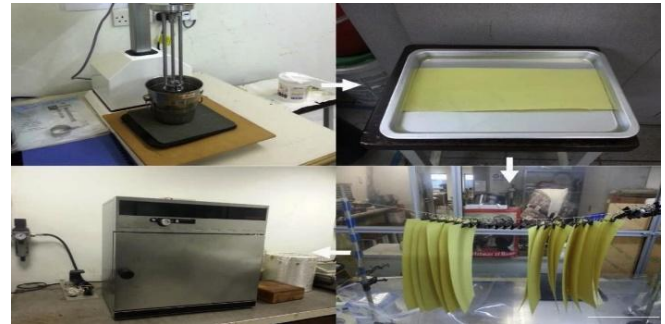
Figure 1. The preparation process of a ballistic fabric sample impregnated in a shear thickening fluid (STF) (Gurgen, Kushan, & Li, 2017)
