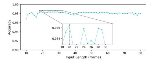
fusion-after-LSTM mechanism. The results are summarized in Fig. 11, which indicates that the 20-frame input length yields better results than other input frame lengths. Therefore, we have selected the 20-frame as  $\Delta$  in Fig. 1, i.e., the input length of our model.
