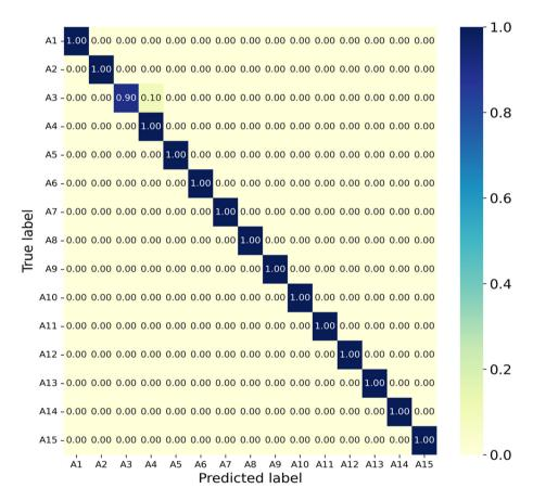
most classification results are concentrated along the diagonal with the accuracy of 100%, showing the high performance of our model, except that 10% of the activity A3 (*check*) is recognized as activity A4 (*connect cables*). The *Accuracy*, *Precision*, *Recall*, and  $F_1Score$  of the model for the 15 activities in Table 5 show the same results, in which all accuracy values are > 99%.
