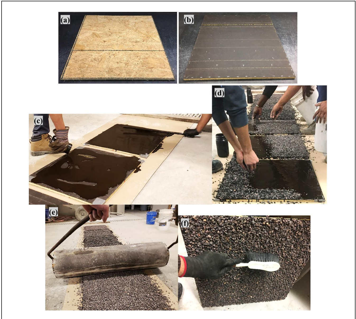
Figure 2. Specimen preparation procedure: (a) plywood base; (b) plywood covered with asphalt felt; (c) pouring and spreading the binder; (d) spreading the aggregate; (e) compaction; and (f) hand brushing before testing.
