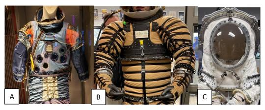
Figure 1.3.-1. Spacesuit Torsos, A: A7L-B Soft Torso Spacesuit, B: NDX-1 Hard Upper Torso Spacesuit, C: Morphing Upper Torso
