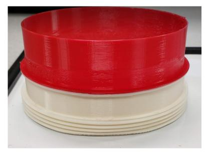
Figure 5.2.2.-1. Dual material 3D printed component, demonstrating the mating of flexible and rigid thermopolymers.
