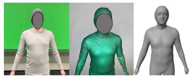
Figure 2.6.1-1. Scan Processing. A: Test subject, B: 3D scan data, C: Ho-model deformed to fit 3D scan data.
