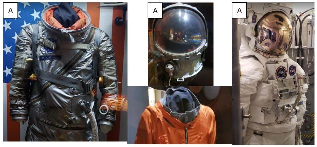
Figure 1.3.2.-2. Alternative suit entry methods, [Left] Mercury spacesuit, with spiral zipper entry [Middle] SK-1 Soviet training spacesuit, with a neck entry method [Right] Shuttle EMU, with a waist entry method.
