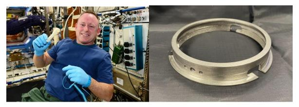
**Figure 5.2.5.-1. 3D Printing in Space Capabilities.** [Left] first object 3D printed in space, a small rachet tool [Right] 3D printed titanium glove disconnect part
