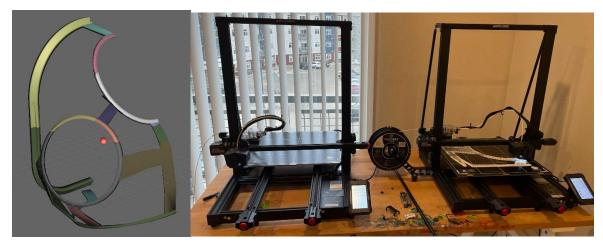
**Figure 5.2.-1. 3D Printed Mockup** Process. [Left] CAD geometry of skeletonized HUT mockup [Right] 3D Printers used to fabricate HUT mockups.
