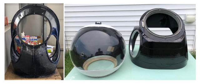
**Figure 5.3.1.-1. 3D Printed HUTs.** [Left] custom sized NDX-4 HUT, featuring a rear entry hatch [Right] NDX-3 HUT, featuring a dual planar entry method
