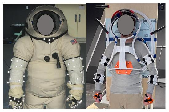
**Figure 4.2.1.-2. IR Motion Capture Tracker Plates.** [Left] suited tracker system [Right] shirt sleeve tracker system.
