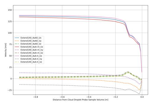
**Figure 39:** Subset of the velocity field through the mesh leading up to the Cloud Droplet Probe sample volume for the Extended Pylon solutions with the boundary conditions of 140 meters per second freestream and all simulated angle of attacks.
