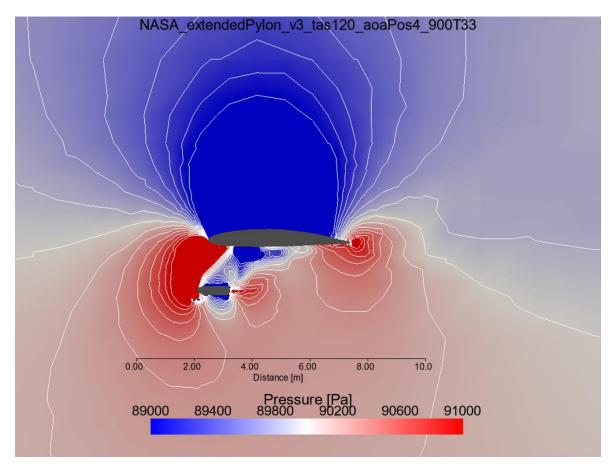
**Figure 32:** NASA P-3 Orion Extended Pylon configuration showcasing velocity Imagnitudes with a two-dimensional slice through the solution with a view point along the lwing (into the page is towards the fuselage). For this simulation, boundary conditions are: freestream airspeed 120 meters per second, angle of attack negative four degrees, freestream 'pressure 900 millibars and temperature 33 degrees Celsius. Contours represent every 3.33 meters per second difference in velocity.
