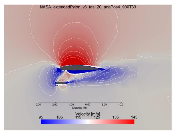
**Figure 30:** NASA P-3 Orion Extended Pylon configuration showcasing velocity magnitudes with a two-dimensional slice through the solution with a view point along the wing (into the page is towards the fuselage). For this simulation, boundary conditions are: freestream airspeed 120 meters per second, angle of attack positive four degrees, freestream pressure 900 millibars and temperature 33 degrees Celsius. Contours represent every 3.33 meters per second difference in velocity.
