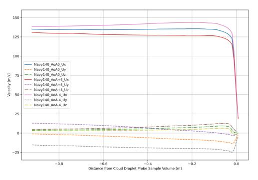
**Figure 37:** Subset of the velocity field through the mesh leading up to the Cloud Droplet Probe sample volume for the Navy Pylon solutions with the boundary conditions of 140 meters per second freestream and all simulated angle of attacks.
