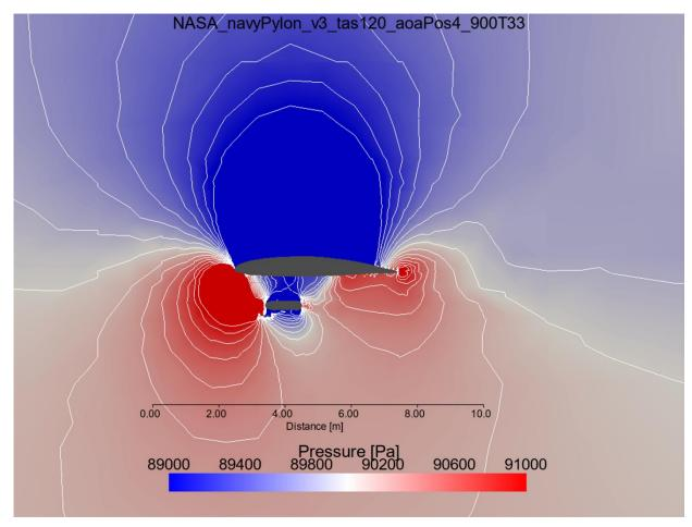
**Figure 23:** NASA P-3 Orion Navy Pylon configuration showcasing atmospheric pressure with a two-dimensional slice through the center line of the Cloud Droplet Probe. For this simulation, boundary conditions are: freestream airspeed 120 meters per second, angle of attack positive four degrees, freestream pressure 900 millibars and temperature 33 degrees Celsius. Contours represent every 133.3 Pa difference in pressures.
