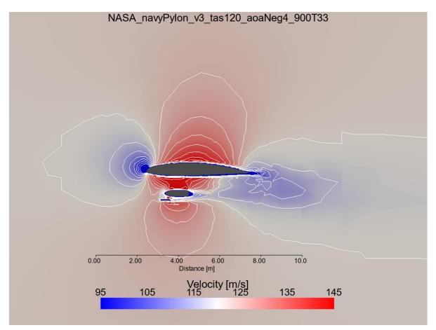
**Figure 24:** NASA P-3 Orion Navy Pylon configuration showcasing velocity magnitudes with a two-dimensional slice through the solution with a view point along the wing (into the page is towards the fuselage). For this simulation, boundary conditions are: freestream airspeed 120 meters per second, angle of attack negative four degrees, freestream pressure 900 millibars and temperature 33 degrees Celsius. Contours represent every 3.33 meters per second difference in velocity.
