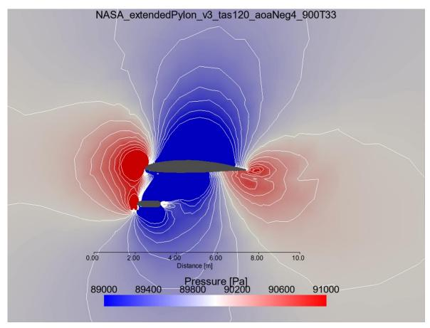
**Figure 33:** NASA P-3 Orion Extended Pylon configuration showcasing atmospheric pressure with a two-dimensional slice through the center line of the Cloud Droplet Probe. For this simulation, boundary conditions are: freestream airspeed 120 meters per second, angle of attack negative four degrees, freestream pressure 900 millibars and temperature 33 degrees Celsius. Contours represent every 133.3 Pa difference in pressures.
