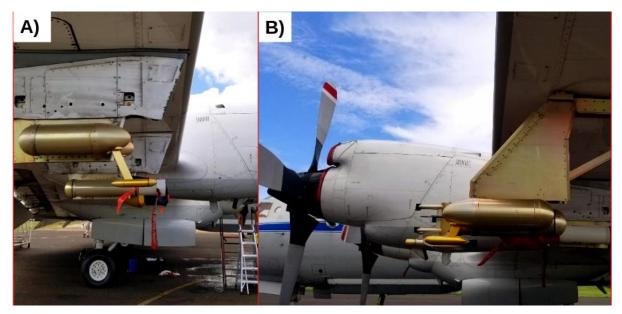
**Figure 4:** Cloud Droplet Probe (CDP) mounting locations with respect to the leading edge of the wings on-board the NASA P-3 Orion during the ORACLES 2018 field experiment in Sao Tome. Figure 1-A (Figure 1-B) contains the Navy (Extended) pylon design with the Langley Airborne Research Center (Uni. Of Hawaii) CDP.
