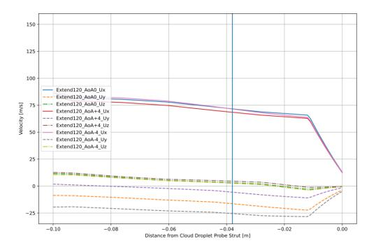
**Figure 41:** Subset of the velocity field through Cloud Droplet Probe sample volume (marked by vertical blue line) for the Extended Pylon solutions with the boundary conditions of 120 meters per second freestream and all simulated angle of attacks.
