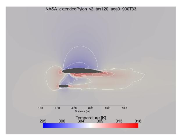
**Figure 29:** NASA P-3 Orion Extended Pylon configuration showcasing total temperature with a two-dimensional slice along centerline of the aircraft fuselage. For this simulation, boundary conditions are: freestream airspeed 120 meters per second, angle of attack zero degrees, freestream pressure 900 millibars and temperature 33 degrees Celsius. Contours represent every 1.5 Kelvin difference in temperature.
