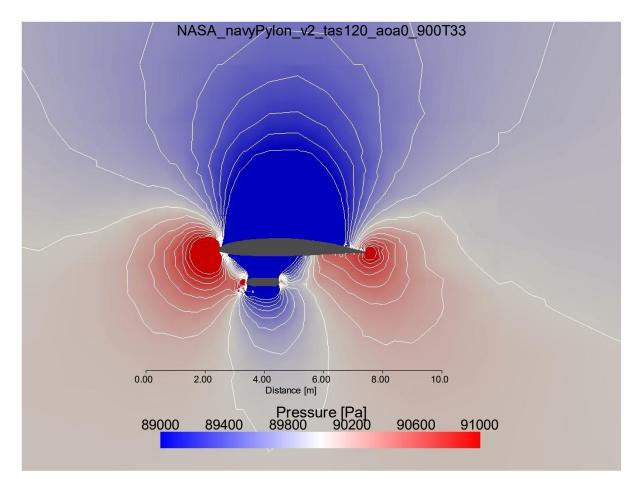
**Figure 16:** NASA P-3 Orion Navy Pylon configuration showcasing atmospheric pressure with a two-dimensional slice through the center line of the Cloud Droplet Probe. For this simulation, boundary conditions are: freestream airspeed 120 meters per second, angle of attack zero degrees, freestream pressure 900 millibars and temperature 33 degrees Celsius. Contours represent every 133.3 Pa difference in pressures.
