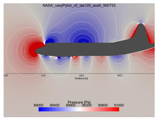
**Figure 18:** NASA P-3 Orion Navy Pylon configuration showcasing atmospheric pressure with a two-dimensional slice through the centerline of the fuselage. For this simulation, boundary conditions are: freestream airspeed 120 meters per second, angle of attack zero degrees, freestream pressure 900 millibars and temperature 33 degrees Celsius. Contours represent every 133.3 Pa difference in pressures.
