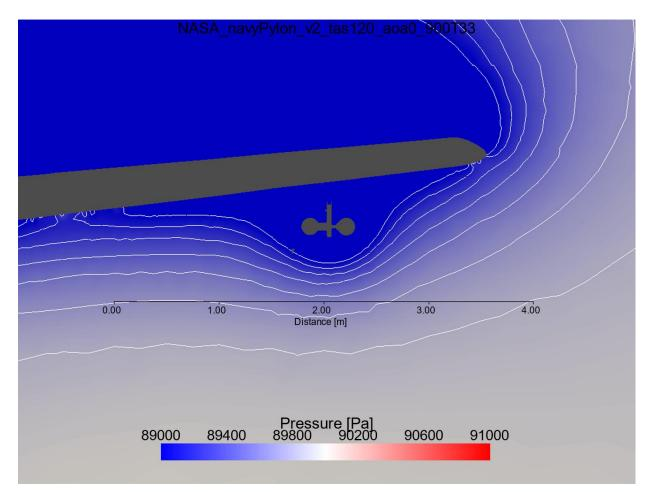
**Figure 17:** NASA P-3 Orion Navy Pylon configuration showcasing atmospheric pressure with a two-dimensional slice across the leading edge of the aircraft wing. For this simulation, boundary conditions are: freestream airspeed 120 meters per second, angle of attack zero degrees, freestream pressure 900 millibars and temperature 33 degrees Celsius. Contours represent every 133.3 Pa difference in pressures.
