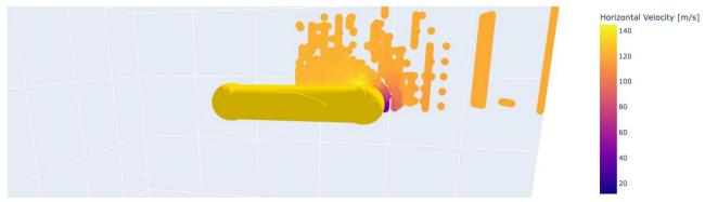
**Figure 43:** Simulated Lagrangian particles (10 micron in diameter, 100 #/cc concentration) for the compressible flow simulation of airflow around a Particle Measurement System canister used during ORACLES. Particles are shaded with calculated horizontal velocities, with a departure from freestream centered in front of the canister.
