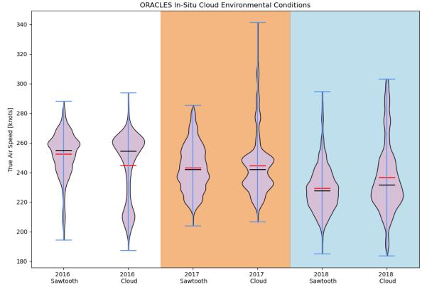
**Figure 10**:True Air Speed for the NASA P-3 Orion during in-situ cloud sampling throughout ORACLES. Shading for each violin plot represents data distribution. Red (black) lines indicate mean (median) of the distribution.
