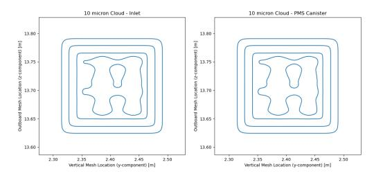
**Figure 44:** Kernel Density Estimation for simulated particles (10 microns, 100 #/cc) within the compressible flow simulation around the Navy Pylon configuration. Left side of figure contains kernel density for the simulation inlet, while right side of figure contains estimate for particles directly in front of the Cloud Droplet Probe canister. Contoured are 99% of all particles.
