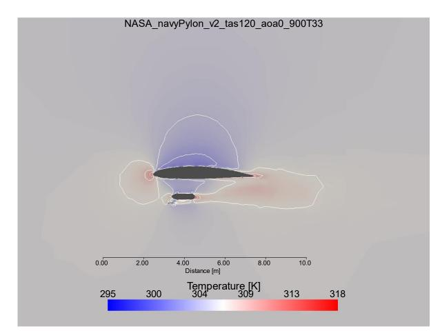
**Figure 19:** NASA P-3 Orion Navy Pylon configuration showcasing total temperature with a two-dimensional slice through the center of the Cloud Droplet Probe. For this simulation, boundary conditions are: freestream airspeed 120 meters per second, angle of attack zero degrees, freestream pressure 900 millibars and temperature 33 degrees Celsius. Contours represent every 1.5 Kelvin difference in temperature.
