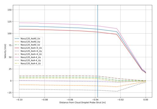
**Figure 40:** Subset of the velocity field through Cloud Droplet Probe sample volume (marked by vertical blue line) for the Navy Pylon solutions with the boundary conditions of 120 meters per second freestream and all simulated angle of attacks.
