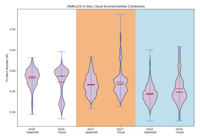
**Figure 7**: Mach Number for the NASA P-3 Orion during in-situ cloud sampling throughout ORACLES. Shading for each violin plot represents data distribution. Red (black) lines indicate mean (median) of the distribution.
