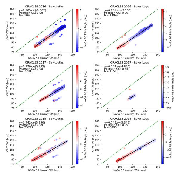
**Figure 47:** Comparison of true air speed observations between the Cloud, Aerosol, and Precipitation Spectrometer and NASA P-3 fuselage. For ORACLES 2016, the Cloud, Aerosol, Precipitation Spectrometer was mounted to the Navy Pylon on the port side outboard pylon. For ORACLES 2017, at the same location, the Cloud, Aerosol, Precipitation Spectrometer was mounted to the Extended Pylon.
