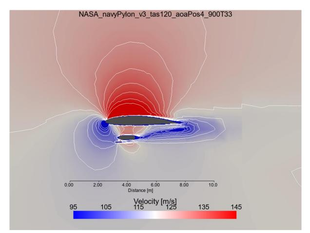
**Figure 22:** NASA P-3 Orion Navy Pylon configuration showcasing velocity magnitudes with a two-dimensional slice through the solution with a view point along the wing (into the page is towards the fuselage). For this simulation, boundary conditions are: freestream airspeed 120 meters per second, angle of attack positive four degrees, freestream pressure 900 millibars and temperature 33 degrees Celsius. Contours represent every 3.33 meters per second difference in velocity.
