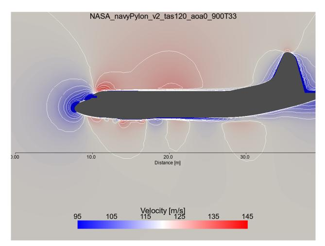
**Figure 15:** NASA P-3 Orion Navy Pylon configuration showcasing velocity magnitudes with a two-dimensional slice through the center line of the fuselage For this simulation, boundary conditions are: freestream airspeed 120 meters per second, angle of attack zero degrees, freestream pressure 900 millibars and temperature 33 degrees Celsius. Contours represent every 3.33 meters per second difference in velocity.
