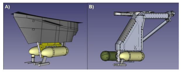
**Figure 5:** Three-dimensional computer-aided design (CAD) models of the NASA P-3 Navy pylon configuration (Figure 2-A) and Extended pylon configuration (Figure 2-B). Each configuration contains designs for the Cloud Droplet Probe and "bullet" canister used during ORACLES 2018.
