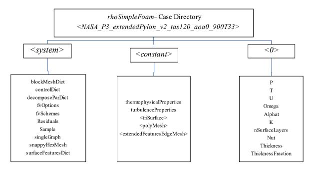
**Figure 11**: Directory structure for the OpenFOAM solver, *rhoSimpleFoam*, for the *NASA\_P3\_extendedPylon\_v2\_tas120\_aoa0\_900T33* case. Listed are all required files for processing. Names listed within brackets indicate a directory.
