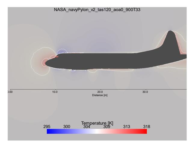
**Figure 21:** NASA P-3 Orion Navy Pylon configuration showcasing total temperature with a two-dimensional slice along centerline of the aircraft fuselage. For this simulation, boundary conditions are: freestream airspeed 120 meters per second, angle of attack zero degrees, freestream pressure 900 millibars and temperature 33 degrees Celsius. Contours represent every 1.5 Kelvin difference in temperature.
