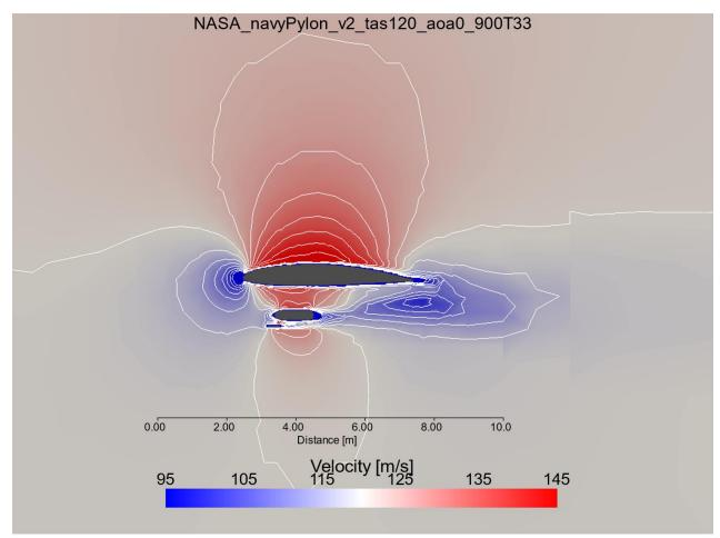
**Figure 13**: NASA P-3 Orion Navy Pylon configuration showcasing velocity magnitudes with a two-dimensional slice through the solution with a view point along the wing (into the page is towards the fuselage). For this simulation, boundary conditions are: freestream airspeed 120 meters per second, angle of attack zero degrees, freestream pressure 900 millibars and temperature 33 degrees Celsius. Contours represent every 3.33 meters per second difference in velocity.
