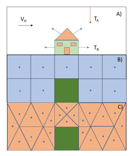
**Figure 3**: Domain discretization for the simplified example of horizontal wind flow across a building (shown in green), with structured (B) and unstructured mesh (C) and associated centroids.
