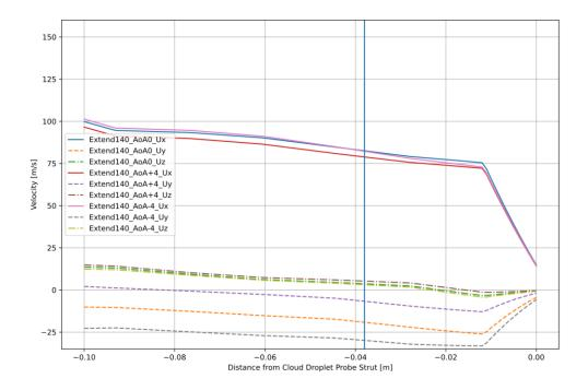
**Figure 42:** Subset of the velocity field through Cloud Droplet Probe sample volume (marked by vertical blue line) for the Extended Pylon solutions with the boundary conditions of 140 meters per second freestream and all simulated angle of attacks.
