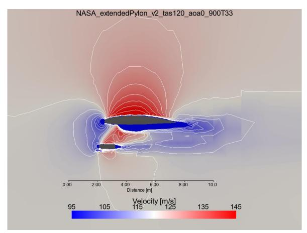
**Figure 26:** NASA P-3 Orion Extended Pylon configuration showcasing velocity magnitudes with a two-dimensional slice through the solution with a view point along the wing (into the page is towards the fuselage). For this simulation, boundary conditions are: freestream airspeed 120 meters per second, angle of attack zero degrees, freestream pressure 900 millibars and temperature 33 degrees Celsius. Contours represent every 3.33 meters per second difference in velocity.
