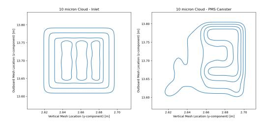
**Figure 45:** Kernel Density Estimation for simulated particles (10 microns, 100 #/cc) within the compressible flow simulation around the Extended Pylon configuration. Left side of figure contains kernel density for the simulation inlet, while right side of figure contains estimate for particles directly in front of the Cloud Droplet Probe canister. Contoured are 99% of all particles.
