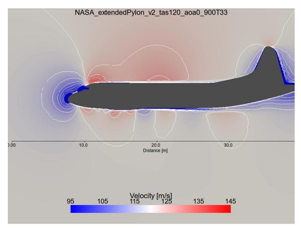
**Figure 34:** NASA P-3 Orion Extended Pylon configuration showcasing airflow velocity with a two-dimensional slice along centerline of the aircraft fuselage. For this simulation, boundary conditions are: freestream airspeed 120 meters per second, angle of attack zero degrees, freestream pressure 900 millibars and temperature 33 degrees Celsius. Contours represent every 3.33 meters per second.
