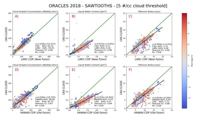
**Figure 48:** Comparison of Cloud and Aerosol Spectrometer with two Cloud Droplet Probes during the sawtooth cloud profiles from ORACLES 2018. Within this figure, New Pylon refers to the Extended Pylon configuration, while Old Pylon refers to Navy Pylon configuration.
