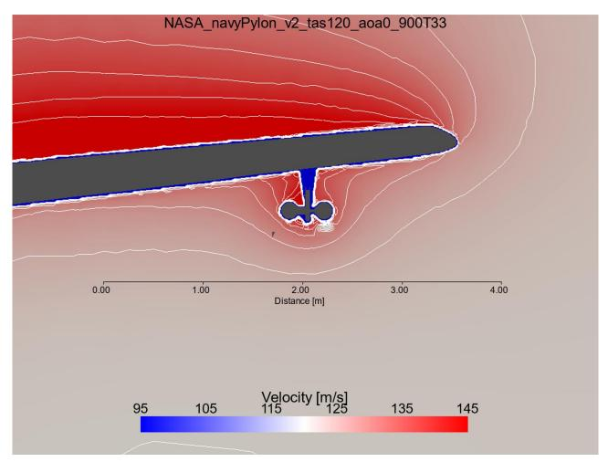
**Figure 14:** NASA P-3 Orion Navy Pylon configuration showcasing velocity magnitudes with a two-dimensional slice through the solution with a view point along the wing (into the page is towards the fuselage). For this simulation, boundary conditions are: freestream airspeed 120 meters per second, angle of attack zero degrees, freestream pressure 900 millibars and temperature 33 degrees Celsius. Contours represent every 3.33 meters per second difference in velocity.
