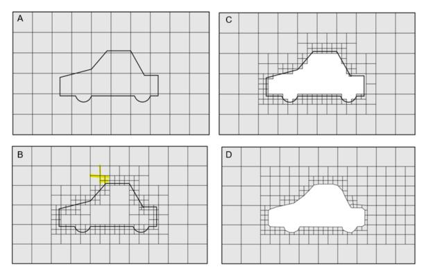
**Figure 6:** Example of the mesh generation from the snappyHexMesh meshing utility, detailing the structure outline (a), splitting of the domain around this structure (b), removal of interior cells (c), and incorporation into the domain (d). Figure is a modification of Figure 5.8, Figure 5.10, Figure 5.11, and Figure.13 within Greenshields 2016).
