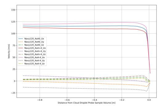
**Figure 36:** Subset of the velocity field through the mesh leading up to the Cloud Droplet Probe sample volume for the Navy Pylon solutions with the boundary conditions of 120 meters per second freestream and all simulated angle of attacks.
