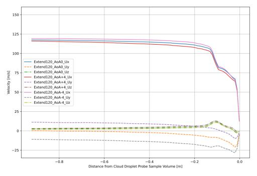
**Figure 38:** Subset of the velocity field through the mesh leading up to the Cloud Droplet Probe sample volume for the Extended Pylon solutions with the boundary conditions of 120 meters per second freestream and all simulated angle of attacks.
