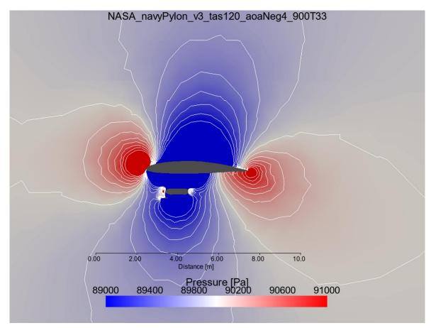
**Figure 25:** NASA P-3 Orion Navy Pylon configuration showcasing atmospheric pressure with a two-dimensional slice through the center line of the Cloud Droplet Probe. For this simulation, boundary conditions are: freestream airspeed 120 meters per second, angle of attack negative four degrees, freestream pressure 900 millibars and temperature 33 degrees Celsius. Contours represent every 133.3 Pa difference in pressures.
