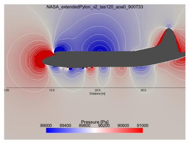
**Figure 35:** NASA P-3 Orion Extended Pylon configuration showcasing pressure field with a two-dimensional slice along centerline of the aircraft fuselage. For this simulation, boundary conditions are: freestream airspeed 120 meters per second, angle of attack zero degrees, freestream pressure 900 millibars and temperature 33 degrees Celsius. Contours represent every 133.3 Pa.
