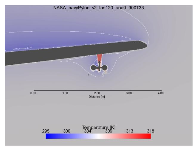
**Figure 20:** NASA P-3 Orion Navy Pylon configuration showcasing total temperature with a two-dimensional slice along the leading edge of the aircraft wing. For this simulation, boundary conditions are: freestream airspeed 120 meters per second, angle of attack zero degrees, freestream pressure 900 millibars and temperature 33 degrees Celsius. Contours represent every 1.5 Kelvin difference in temperature.
