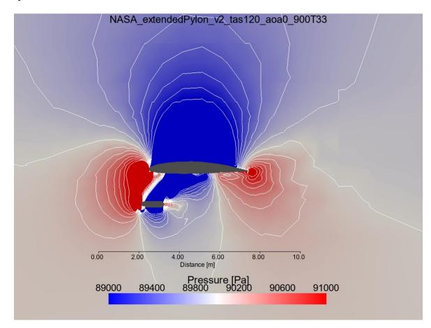
**Figure 28:** NASA P-3 Orion Extended Pylon configuration showcasing atmospheric pressure with a two-dimensional slice through the center line of the Cloud Droplet Probe. For this simulation, boundary conditions are: freestream airspeed 120 meters per second, angle of attack zero degrees, freestream pressure 900 millibars and temperature 33 degrees Celsius. Contours represent every 133.3 Pa difference in pressures.
