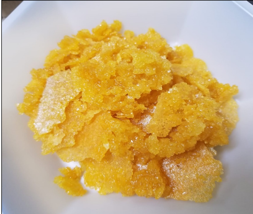
Figure 5.20: Salt precipitates of Lindy34-10 (Y) at 430°C - 480°C.
