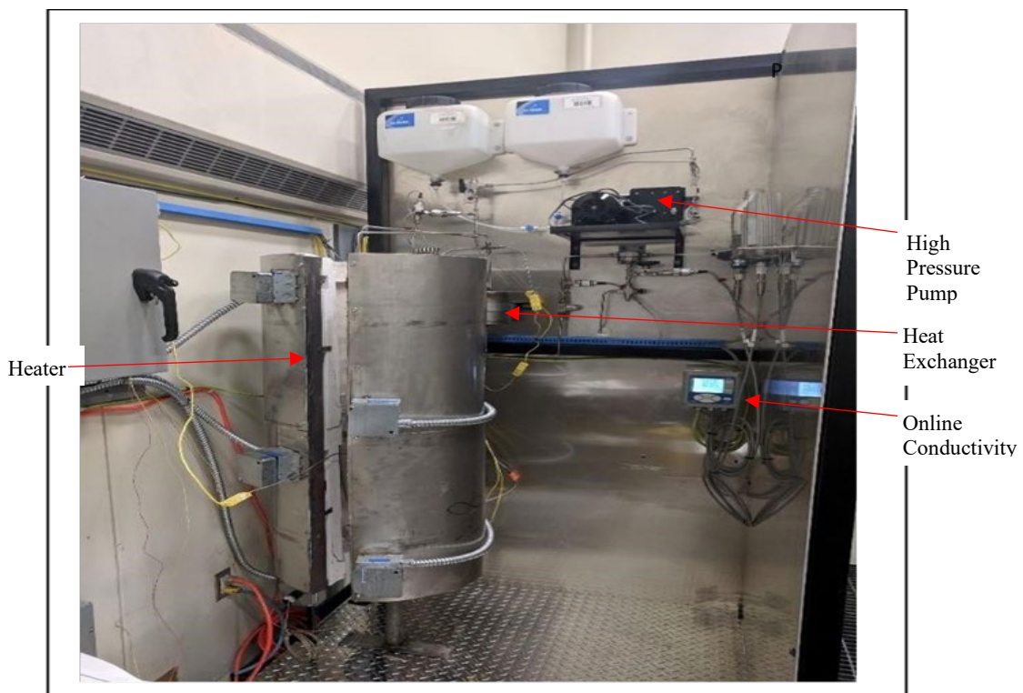
Figure 4.2: Photo of the SCWD Lab-scale setup.
