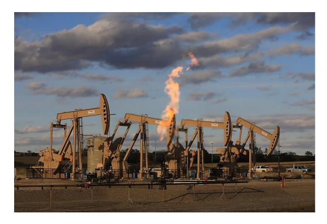
**Figure 7.4.** 'Typical' Bakken Field surface activities. Note multiple wells on pump and central flare. From Cameron, 2021.
