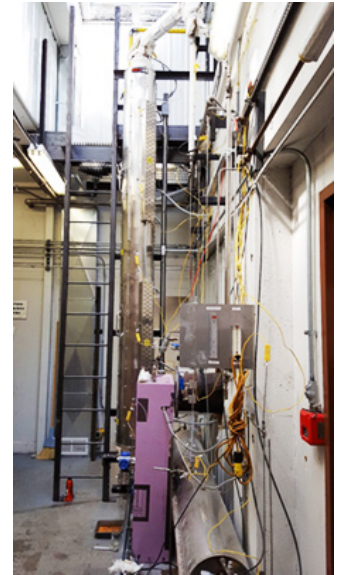
Schematic and photo of the dynamic corrosion test system.
