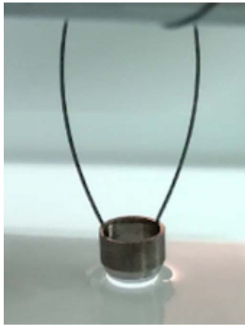
Figure 2. A photo of the ring at the moment of its detachment from the water surface. It shows the deformation of the elastic film formed by the water at the liquid–air interface.
