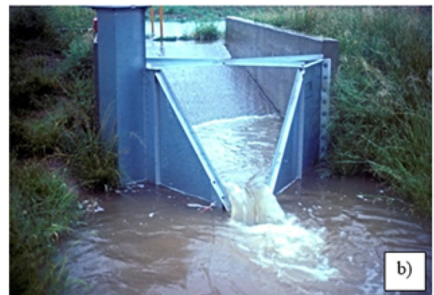
Fig. 1 Sketches (a) and view (b) of a H-flume
