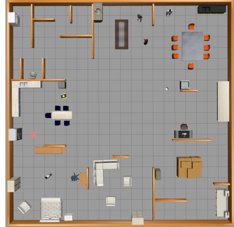
Fig. 3: Example of indoor environment in Gazebo where navigation policies can be trained or tested, accessing different areas with realistic obstacles and narrow passages. A Jackal UGV has been spawned to reach the goal (red circular target).
