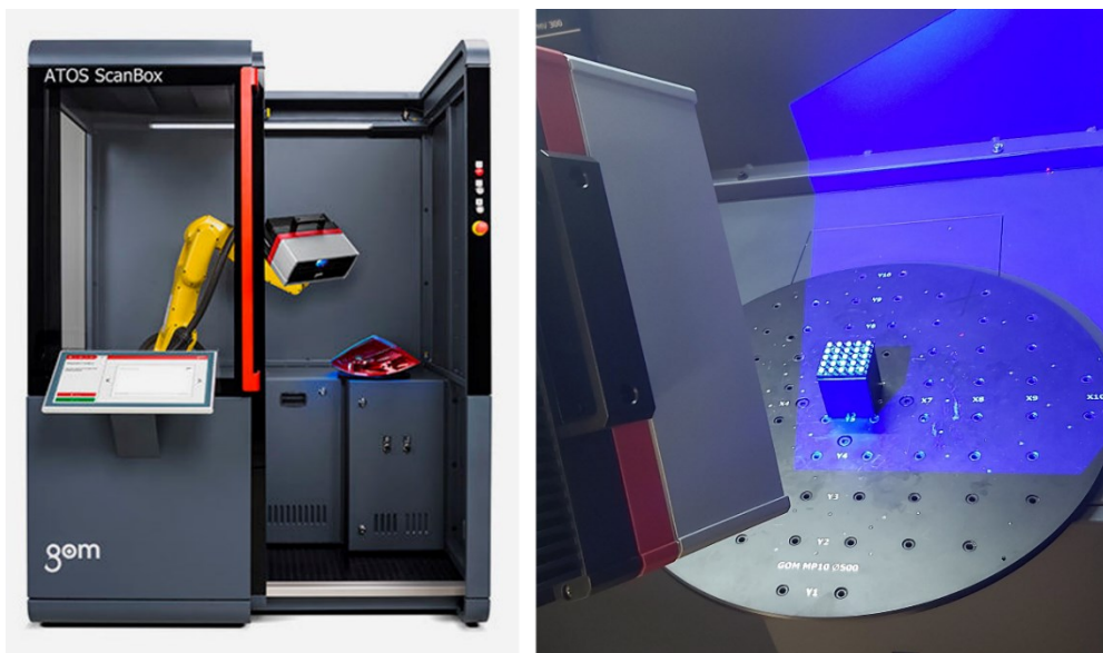
Figure 3.4: Atos ScanBox and a detail of the projected narrow-band blue light from the instrument head on the ball plate positioned on the rotating stage.
