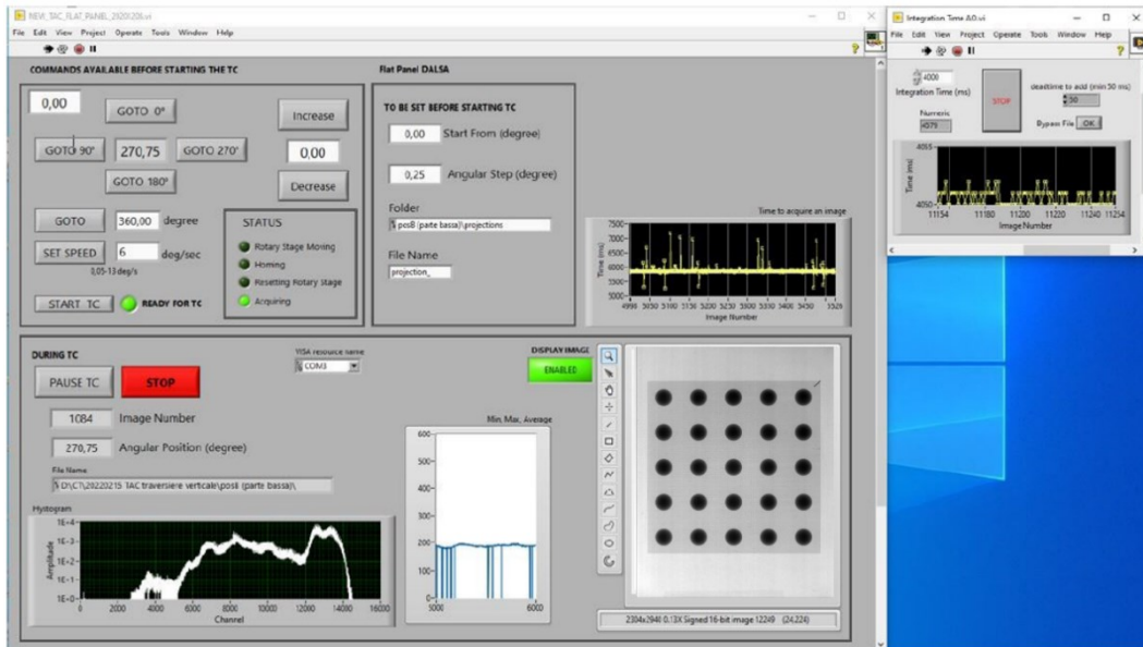
Figure 3.6: LabVIEW program for CT acquisition (main window for setting CT acquisition parameters and minor window for setting of integration time)
