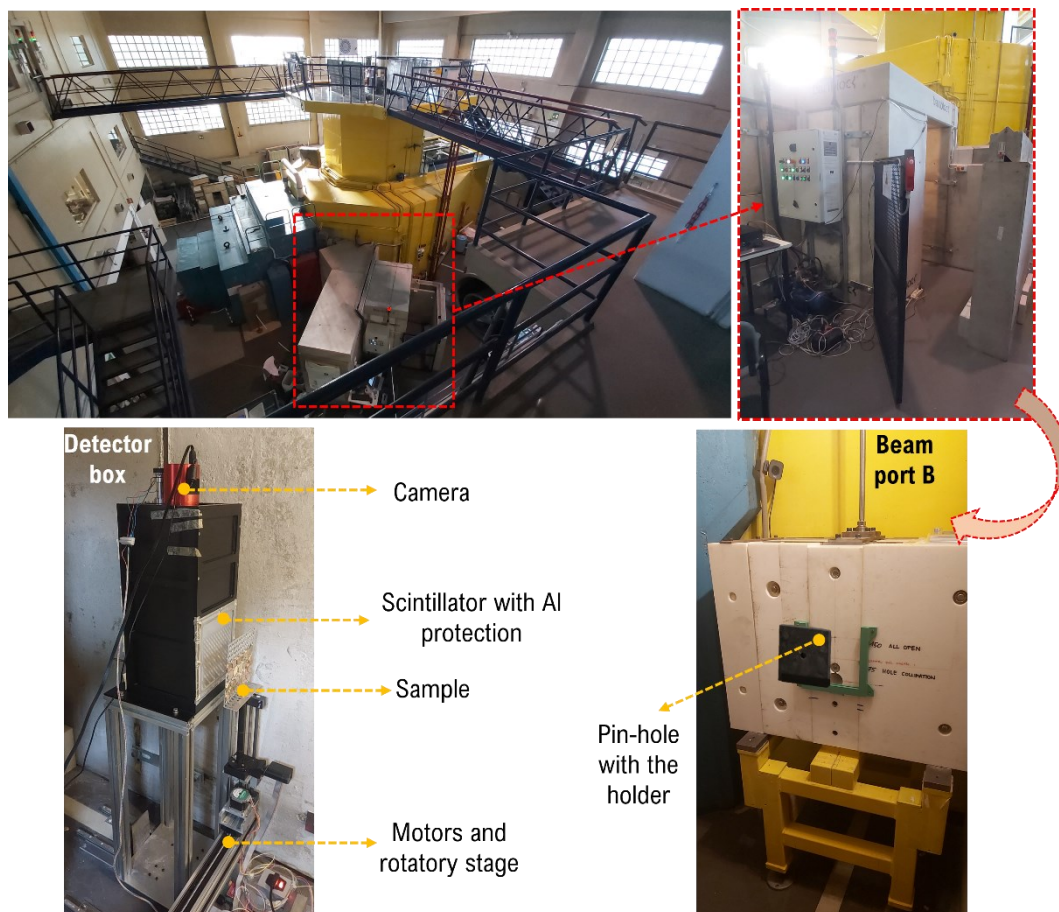
Figure 5.26: The LENA reactor (PV) and the installed NICHE setup in the shielded room. Neutron channel with pinhole and custom-made camera box for imaging analysis is shown.
