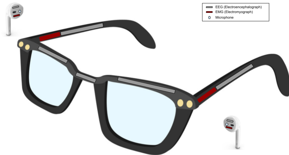
Figure 1: Silent speech interfaces for future AR glasses and hearables embedded with EEG, surface EMG electrodes. The glasses and hearable can be used independently or can also be used together.
