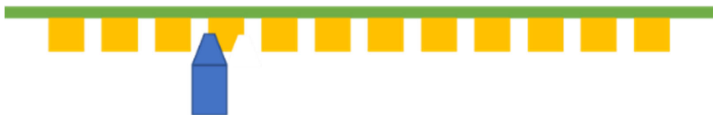
Figure 12: Step 8 – Drilling Left Side of PKG Cu Pillar
