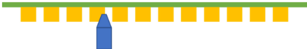
Figure 10: Step 6 – Drilling Right Side of PKG Cu Pillar
