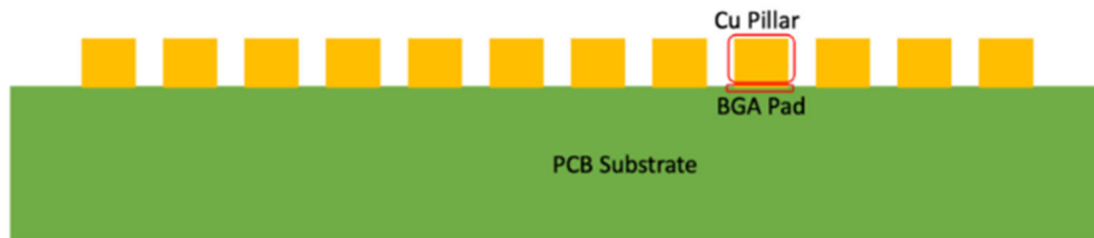
Figure 5: Step 1 – Electroplating PCB BGA Pads
