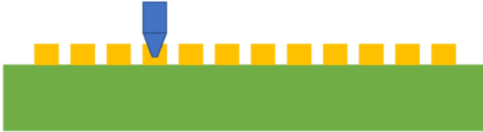
Figure 6: Step 2 – Drilling PCB Cu Pillar
