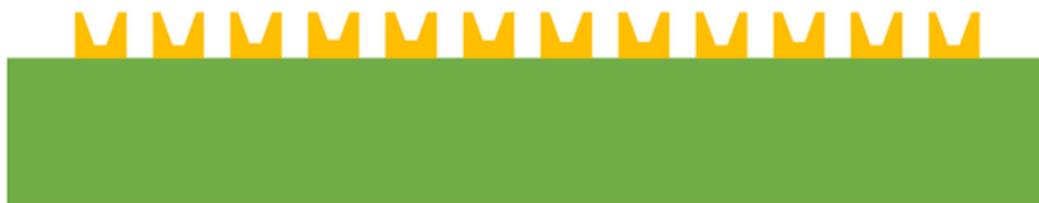
Figure 8: Step 4 – Shaped PCB Cu Pillars
