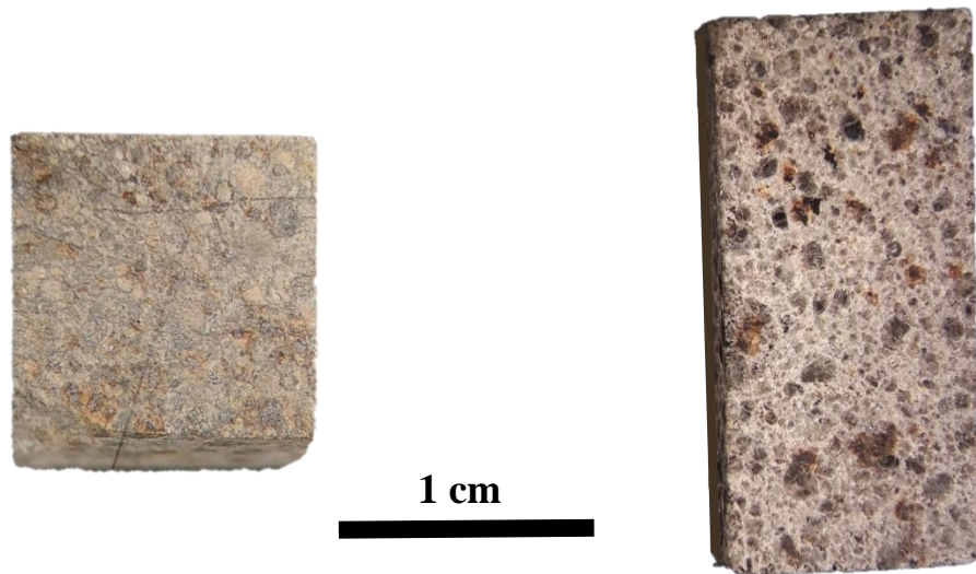
Figure 2.2: example of a Buzzard Coulee cube (on the left) and a cuboid (on the right) of Golden meteorite.
