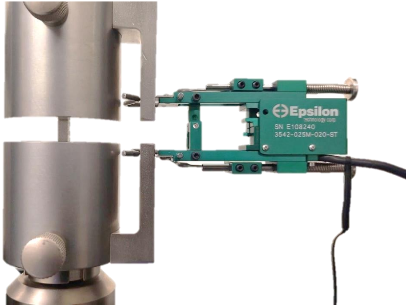
Figure 2.8: The diagram illustrates the extensometer affixed to tabs using knife edges. This configuration enables the precise measurement of strain on very small samples. The depicted sample, an Aluminum alloy positioned between the platens in the image, serves as the designated calibration check standard material.
