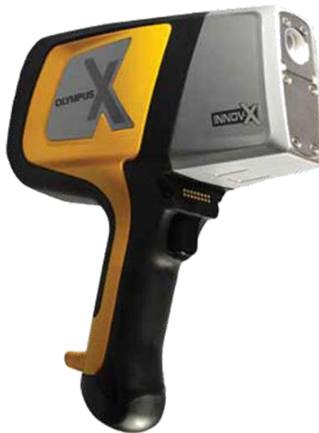
Figure 2.11: The image shows the Olympus® Delta Premium portable ED-XRF analyzer used to measure elemental compositions in this study.
