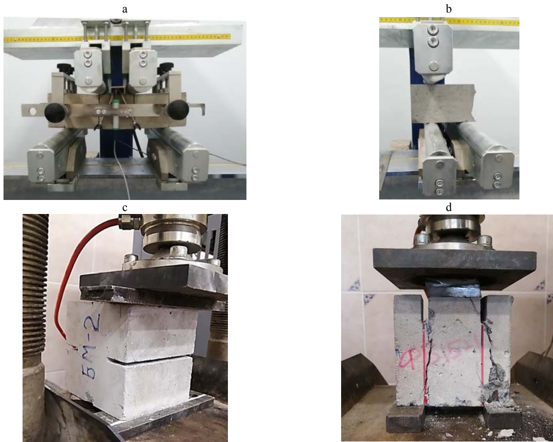
Fig. 6. Tests of nanofibre concrete in laboratory conditions: a – tensile in bending with registration of the fracture diagram; b – tensile during splitting; c – normal separation under eccentric compression; d – transverse shear
