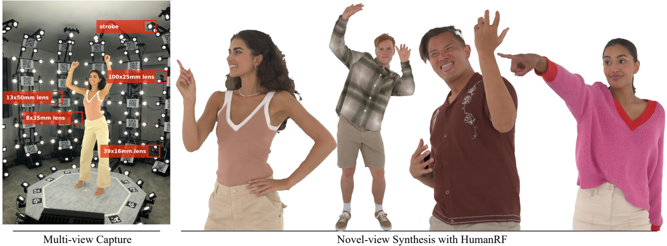
Fig. 1. We introduce a novel multi-view dataset of humans in motion captured with a rig of 160 cameras, recording footage of 12MP each (left image). From an input multi-view recording of a specific person, our HumanRF method reconstructs a spatio-temporal radiance field which captures appearance and motion of the actor. From this representation, we can then synthesize highly-realistic images from unseen, novel view points (right images).
