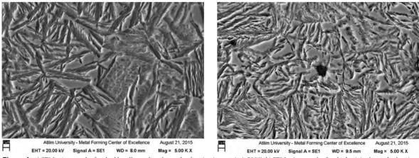
Figure 4. .a) SEM micrograph of etched locally produced sample, showing its matrix (x5000), b) SEM micrograph of etched original sample showing its matrix (x5000)
