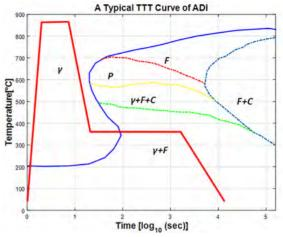
Figure 1. Schematic representation of TTT and a typical heat treatment cycle of ADI (adapted from [23])
