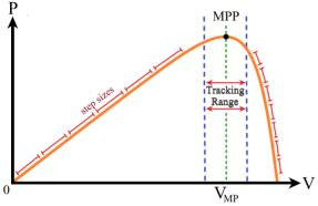
Figure 11. P-V curve of perturb and observe algorithm
