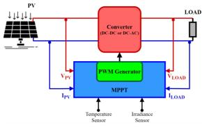
Figure 4. Operating scheme of the MPPT system [10]
