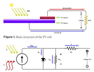
Figure 2. Equivalent circuit of PV cell
