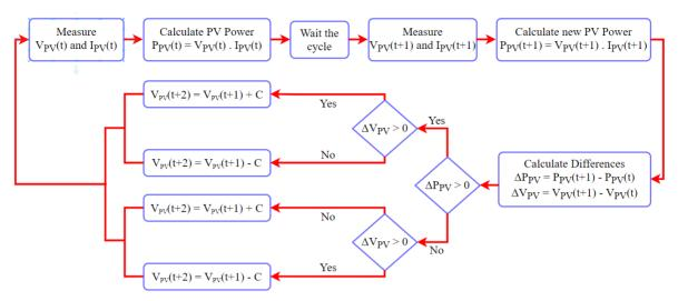
Figure 10. Perturb and observe flowchart
