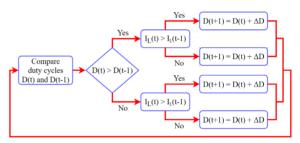
Figure 9. PV output senseless flowchart
