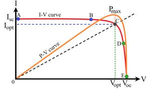
Figure 3. Typical current-voltage characteristics of the PV cell
