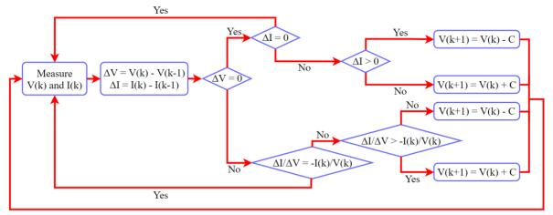
Figure 16. Incremental conductance flowchart
