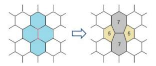
Figure 5. Schematic model showing the transformation of four adjacent hexagons into STW defect
