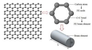
Figure 1. FE modeling of graphene
