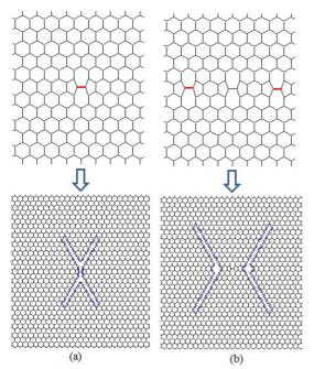
**Figure 8.** Fractured profile of the one (left) and multiple STW-defected GS (tilting angle of  $0^*$ ) (right) under tension
