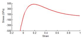
Figure 4. Stress- strain curve of C-C bond
