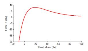
Figure 2. Force-strain curve of modified Morse interatomic potential
