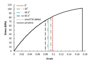
Figure 6. Tensile stress-strain curves of GSs having STW-defects
