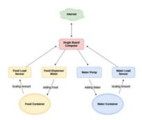
Figure 2. Performing Unit components and flow diagram of the designed IoT.
