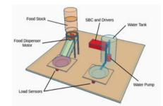
Figure 3. Design sketch of the Performing Unit.
