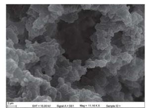
Figure 3. SEM image of poly(HEMA-MATrp) cryogels.
