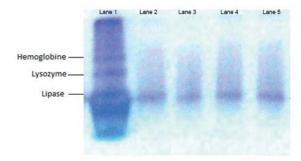
**Figure 12.** SDS-PAGE image for lipase enzyme desorbed from *Candida cylindracea*. Lane 1: Marker (Lipase, Lysozyme, Hemoglobine) Lane 2: Lipase marker, Lane 3: Initial lipase solution [(Before adsorption for Cu nanoparticle embedded poly(HEMA-MATrp) cryogels], Lane 4: Final lipase solution [(After adsorption for Cu nanoparticle embedded poly(HEMA-MATrp) cryogels], Lane 5: Desorbed sample [(After desorption from Cu nanoparticle embedded poly(HEMA-MATrp) cryogels].
