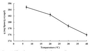
Figure 9. Effect of temperature on the adsorption of lipase enzyme onto Cu nanoparticles embedded cryogels. pH: 6.0 interaction time: 30 min.,  $C_{\rm lipase}$ : 1.5 mg/mL.
