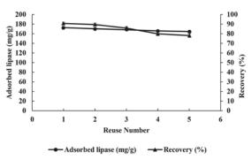
**Figure 11.** Reusability of Cu nanoparticle embedded poly(HEMA-MATrp) cryogels. pH: 6.0, interaction time: 30 min., C<sub>lipase</sub>: 1.5 mg/L, T: 25°C.
