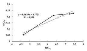
Figure 14. Freundlich adsorption isotherm plotted from experimental values.
