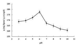
**Figure 6.** Effect of pH on the adsorption of lipase enzyme onto Cu nanoparticles embedded cryogels.  $C_{\rm lipase}$ : 1.5 mg/mL, Interaction time: 30 min., T: 25°C.
