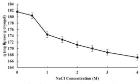
**Figure 10.** Effect of ionic strength on the adsorption of lipase enzyme onto Cu nanoparticles embedded cryogels. H: 6.0, interaction time: 30 min.,  $C_{\text{lipase}}$ : 1.5 mg/mL, T: 25°C.
