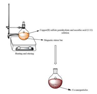
Figure 1. Schematic diagram for Cu nanoparticle synthesis.
