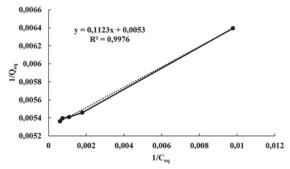
Figure 13. Langmuir adsorption isotherm plotted from experimental values.
