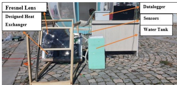
Figure 4. Experimental setup of the designed system
